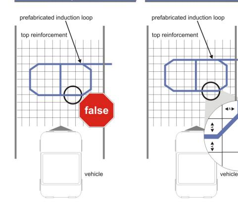
The distance Abetween the prefabricated induction loop and the iron armoring must be equally and as great as possible!
